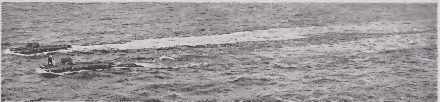
FIGURE 13. Use of bow curtain and stern tarpaulin on experimental DUKW (lower), Woods Hole, Massachusetts.
